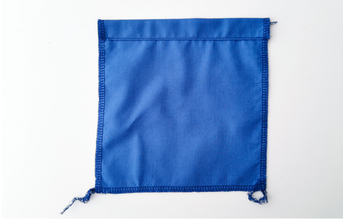
07. Iron a 1cm fold to the upper edge of the patch pockets, press a second fold 2cm and topstitch 2mm from this fold.
