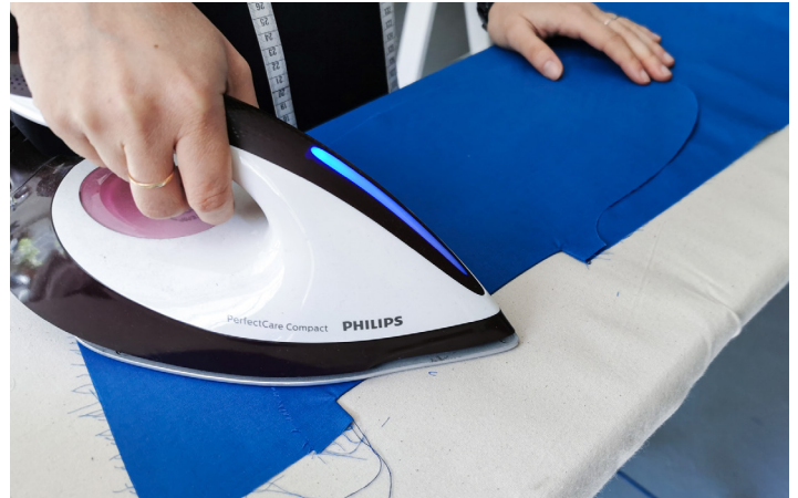
04. Turn the pocket bag to the inside and press, ensuring you get the corners laying flat. If they aren't, you haven't snipped in far enough.
