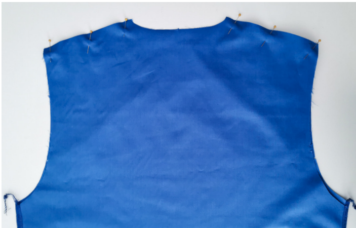
11. With right sides together, sew the front to the back at the shoulder seams, overlock together and press to the back.
