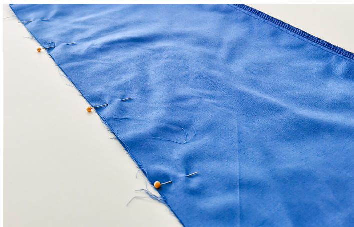
21. Pin the inside leg seams together. Sew and overlock. Press to the back. Repeat on other side.
