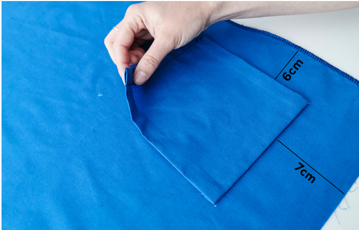
09. Pin the patch pockets to the right side of the front where marked on the front pattern piece. (7cm up from hem edge and 6cm in from side)
