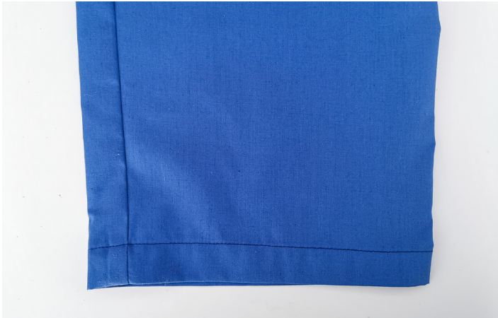
25. Press the hems to the inside 1cm and then 2cm and topstitch.
