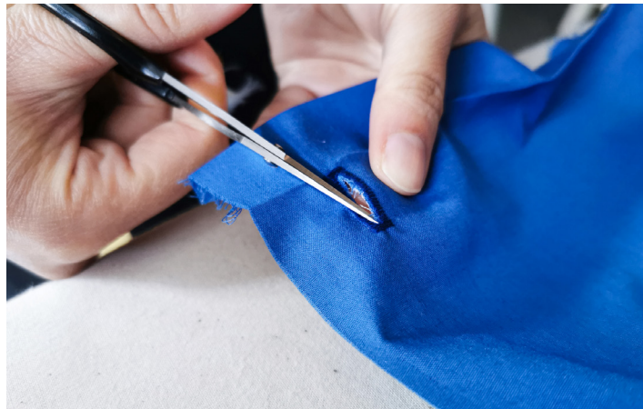
20. Cut the button holes open, taking care not to snip through the end bar tacks.
