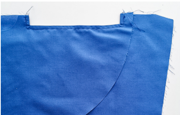
05. Top stitch around the hand opening of the pocket, 2mm from the edge.
