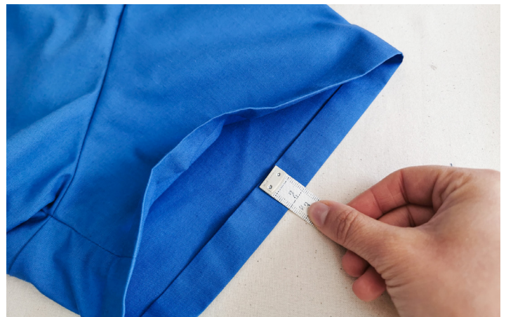
24. Press the sleeve hems up 1cm and then 2cm and topstitch 2mm from the fold. Well done - the top is finished, you are half way there. Just the trousers to go!
