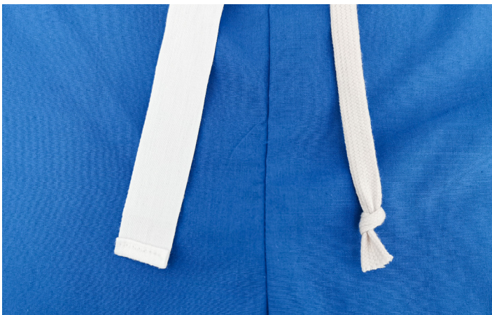
28. Drawstring ends if using tape should be double turned and stitched. Or if you are using cord, ends should be knotted.
