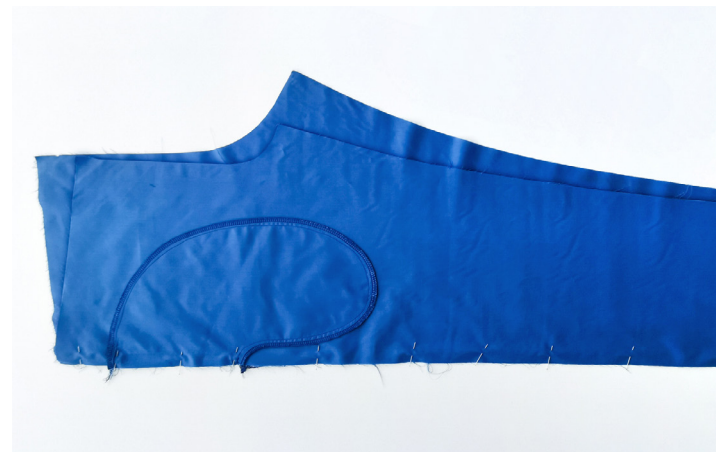
12. Lay the front and back legs right sides together, and pin down the outside leg seam. Match up the pocket openings in the side seams on the front with the corresponding notches on the back.
