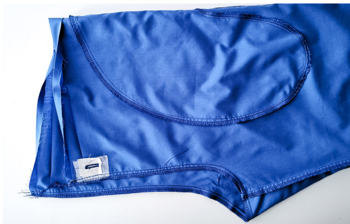
23. Sew the crotch. Then sew the crotch again over the same stitch lines. The crotch is always the first seam to go on a pair of trousers so it is always useful to sew the crotch twice! Overlock the crotch together.
