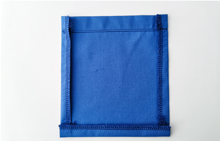
09. Press the marked seam allowance (1.5cm) to the inside of the sides and bottom of the patch pockets.
