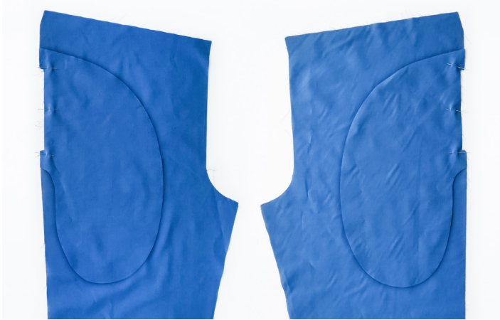
01. With right sides together, align the pocket bag that has the cut out section onto the front leg and pin in place. It is best to do this at the same time to make sure you get a pair and not two lefts!
