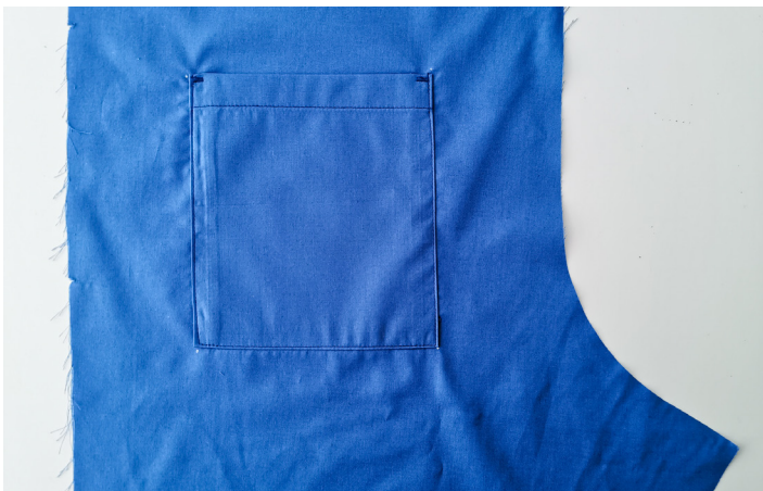
11. Stitch 2mm from the folded edge around the sides and bottom. Bar tack at the top as shown in the photo, or sew a triangle stitch to reinforce the opening.
