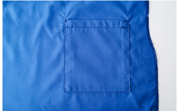
10. Stitch 2mm from the folded edge around the sides and bottom. Bar tack at the top as shown in the photo, or sew a triangle stitch to reinforce the opening.
