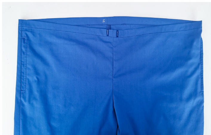
24. Press the waist channel back into position (you should already have a good fold there) embroider size if you are doing so, then topstitch. Insert size label at centre back under channel stitch if you are using a label.
