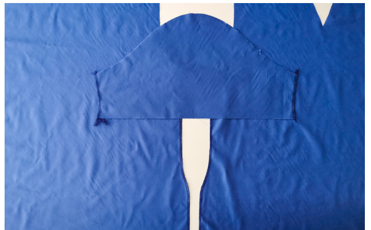
06. Overlock the following seams on the following pieces: Underarm seams of the sleeves, side seams of the front and back (curve off the point as you overlock), sides and bottom of the patch pockets.
