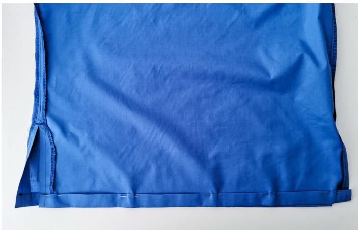
23. On the front, press the hem up 1cm and then 2cm and topstitch 2mm from the fold. Do the same on the back.
