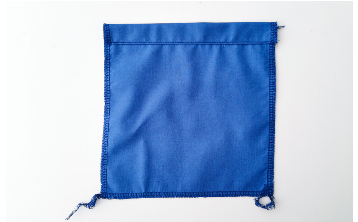
08. Overlock around sides and bottom of patch pockets. Iron a 1cm fold to the upper edge of the patch pockets, press a second fold 2cm and topstitch 2mm from this fold.
