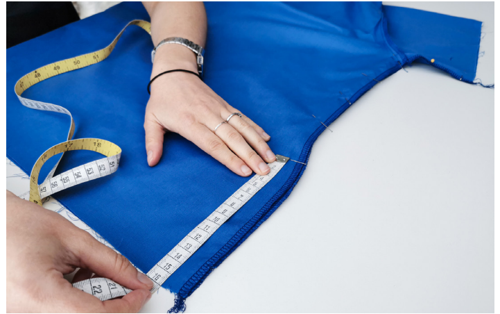
20. With right sides together, sew the side seams along the underside of the sleeve and down to the top of the split on the body. Split should measure 16cm up from the raw hem edge of the front and back on all sizes.
